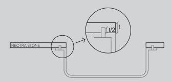
All incisions, slits or drills must pass through the material a maximum of half of the thickness.
