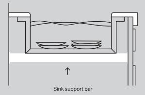
Furthermore, for large sinks, we recommend placing support bars under the sink, so that its weight is borne by the bars and not (by) the worktop.
