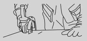
All products of Neotra can be cut using diamond discs fitted onto the hand-held electrical grinding machine. In this case, the SLAB will have a cleaner and better defined edge than by cutting and breaking the SLAB.
