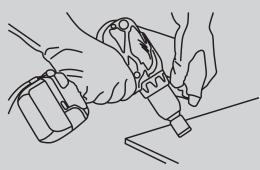
As an alternative, you can use cutting disc fitted to angle grinders, electrical drills or battery-operated screwdrivers.
