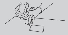
To make rectangular holes in stone, start by making a round hole at each corner of the rectangle. Then make straight cuts between each hole with a discs cutter with a diamond discs. This will prevent excessive stresses being generated at the corners of the rectangle which could then form a crack in the stone itself.
