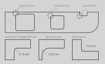
A minimum of 4mm radius is mandatory for inside corners except for L Shapes, where 10 mm is required. Above are recommended examples of cut-outs for fittings such as sinks, hobs, columns, etc.
